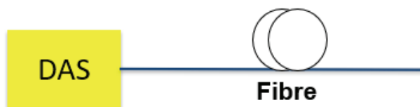
Figure 3, Distributed Acoustic Sensing (DAS) typically uses a separate fibre, but may also be combined with a data transmission system if a separate wavelength band is applied for the DAS system.
