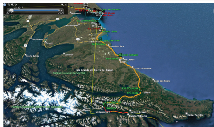
Figure 7: Underground fiber optic network Island Tierra del Fuego, Argentina
