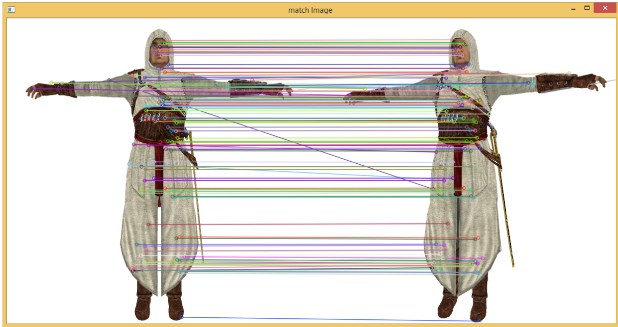
Figure 4.1: Illustrating feature extraction process - detection, description and matching, between stereo pairs.
