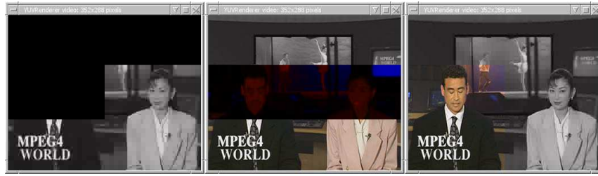
Fig. 6. Screenshots of three video receivers with different subscriptions, illustrating the effect of selecting: (left) only luminance, lowest quality and only some regions, (middle) only luminance, only chrominance, and full quality color for different rows, and (right) only luminance and low quality, except for a region having full quality and colors.
