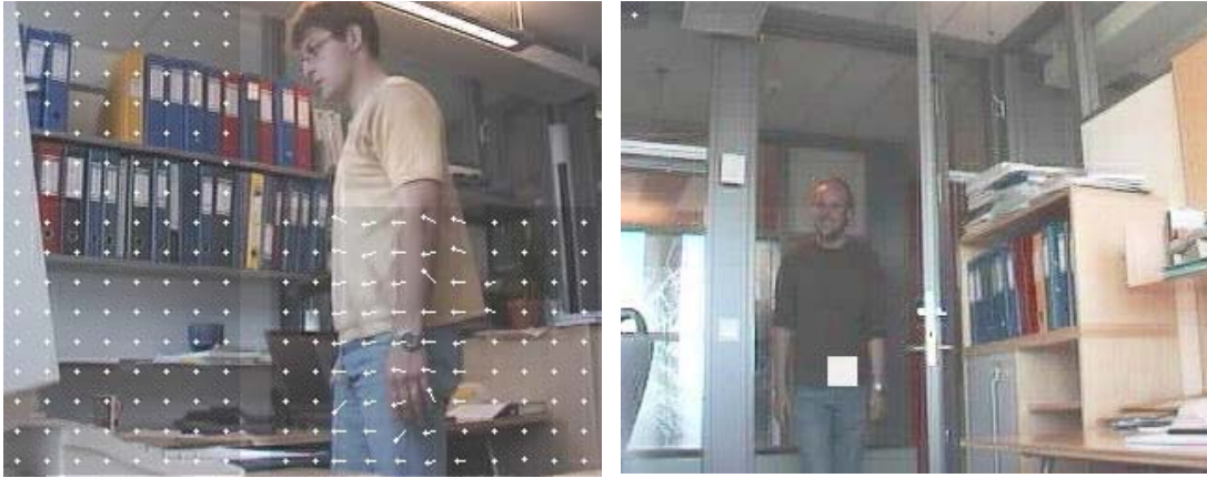
Fig. 3. Left: Block-based motion estimation example. Right: The center position of the tracked object, calculated by the coordinator, has been drawn as a white rectangle
