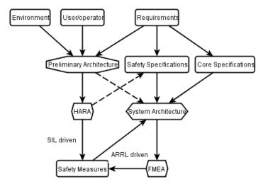
Fig. 2. Simplified view on HARA and FMEA correspondence with SIL and ARRL
