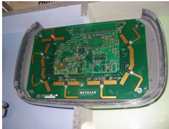
Figure 5.1: The Netgear RangeMax MIMO pre-802.11n wireless access point is able to configure the seven embedded circuit-board arrays into one of 127 different beam patterns.
