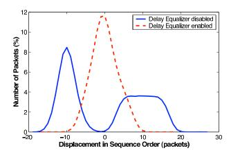
Fig. 9. Buffering packets at the proxy is able to considerably reduce IP packet reordering even if the used links exhibit variable delays.
