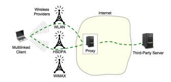
Fig. 1. A multilink proxy is used to schedule traffic from a server to all available interfaces on a client, which is simultaneously connected to a WLAN and an HSDPA access network.
