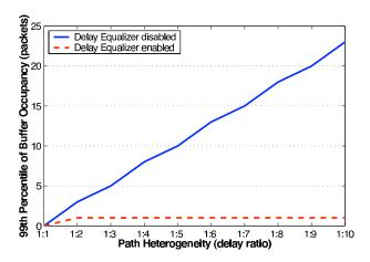
Fig. 8. Reducing IP packet reordering – At the proxy, a buffer is used to delay packets over the low-latency link by putting them into a buffer. This is useful to compensate for latency differences and to reduce the client workload.
