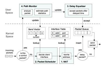
Fig. 4. Internals of the multilink proxy – The destination address of incoming packets is rewritten according to a weighted round-robin schedule. Latency differences are equalized by queuing packets destined to travel over a fast path. Dynamic adaptation to differences in throughput and delay is facilitated through path monitoring feedback from the client.
