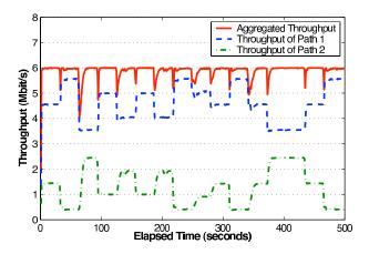
Fig. 7. Adaptive bandwidth aggregation – A send vector based on path monitoring feedback is able to adapt to arbitrary bandwidth changes. In this example, the bandwidths of Link 1 and Link 2 always sum up to 6 Mbit/s.
