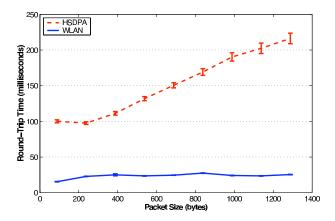
Fig. 2. The heterogeneity of round-trip times is one of the most dominant challenges when aggregating wireless links, such as HSDPA and WLAN. In truly heterogeneous environments, varying the packet size has negligible effect on equalizing the latency of multiple links.
