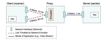
Fig. 6. Multilink test network – The *netem* tool is used to emulate link heterogeneity (bandwidth and latency) in a controlled manner.
