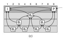
Figure 1: Bitstream dependency examples: (a) Typical MPEG-1/2/4 structure. (b) Layered H.264/AVC structure. (c) Dyadic-tree structure for temporal scalability.
