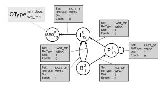
Figure 2: Type dependency graph for a simple MPEG-like stream.
