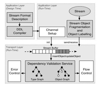
Figure 4: Cross-Layer design using the dependency validation service.
