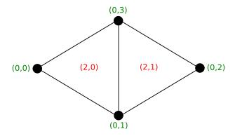
Figure 3: The mesh connectivity  $2 \to 0$  (the vertices of each cell) for this triangular mesh with two cells and four vertices is stored as two arrays indices = [0, 1, 3, 1, 2, 3] and offsets = [0, 3, 6].
