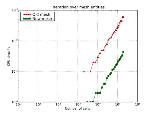
Figure 14: Benchmarking the CPU time for iteration over the vertices of each cell for the new mesh library vs. the old DOLFIN mesh library.
