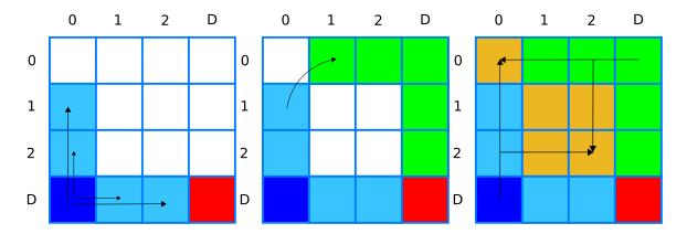
Figure 4: The three basic algorithms for computing connectivity. From the left: Build (computing connectivity  $D \to d$  and  $d \to 0$  from  $D \to 0$  and  $D \to D$ ), Transpose (computing connectivity  $d \to d'$  from  $d' \to d$ ) and Intersection (computing connectivity  $d \to d'$  from  $d \to d''$  and  $d'' \to d'$ ).
