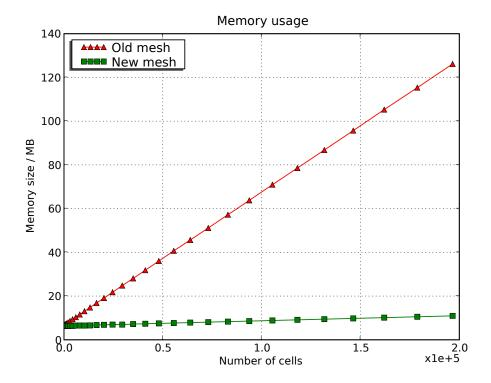
Figure 13: Benchmarking the memory usage for creation of a uniform tetrahedral mesh of the unit cube for the new mesh library vs. the old DOLFIN mesh library.
