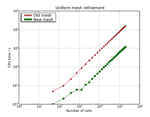
Figure 15: Benchmarking the CPU time for uniform refinement of the unit cube for the new mesh library vs. the old DOLFIN mesh library.
