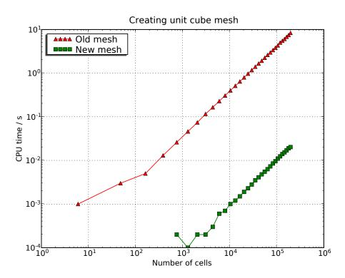
Figure 12: Benchmarking the CPU time for creation of a uniform tetrahedral mesh of the unit cube for the new mesh library vs. the old DOLFIN mesh library.
