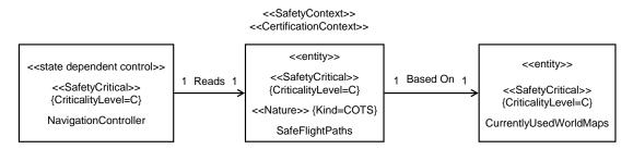
Figure 17: Aircraft's navigation controller using COTS software (structure).
