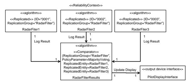
Figure 20: Multiple-version radar filter system (structure).
