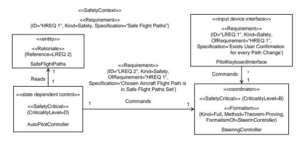
Figure 19: Safety-requirements for an aircraft steering system (structure).
