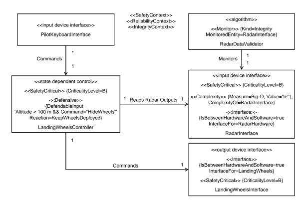
Figure 9: Landing wheel controller processing user and radar inputs (structure).
