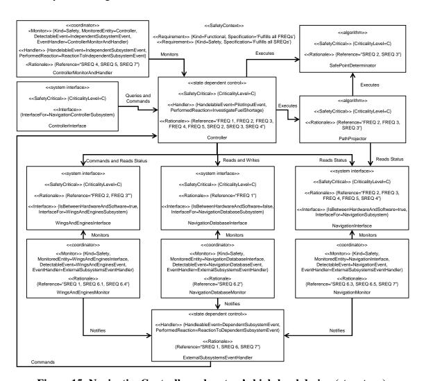
Figure 15: NavigationController subsystem's high-level design (structure).
