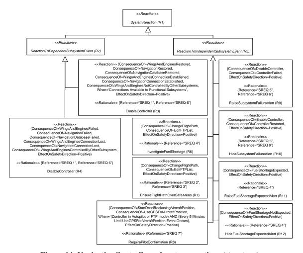
Figure 14: NavigationController subsystem reactions (structure).
