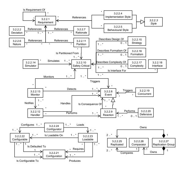
Figure 7: Meta-model for the refined safety-related concepts.
