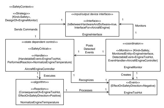
Figure 22: Monitoring the aircraft's engine's temperature (structure).
