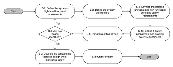
Figure 11: Development methodology of airworthiness-compliant software products.
