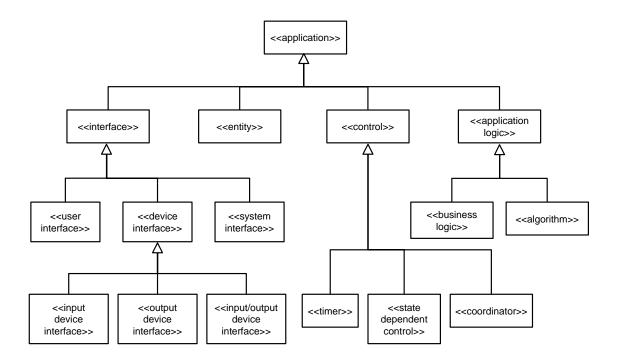
Figure 16: Gomaa's classification of application classes using stereotypes [7].
