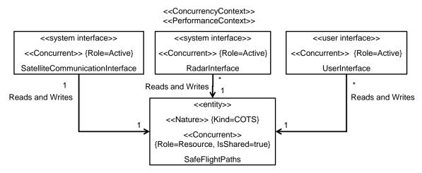
Figure 21: Concurrent access to an aircraft's COTS software (structure).
