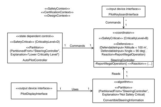
Figure 18: Aircraft steering controller (structure).
