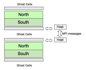
**Figure 2:** North-south computation allows asynchronous communication, thus hiding latency.
