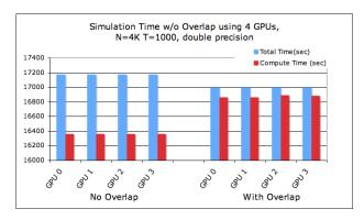
**Figure 4:** Comparison of simulation time w/o overlapping of communication and computation.
