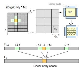
**Figure 1:** Stencil computation on a 2D grid and its memory access pattern. Data and thread block decomposition of  $N_x \times N_y$  input mesh. The mesh is divided into  $d_x \times d_y$  tiles. Each CUDA thread processes a column in a tile.
