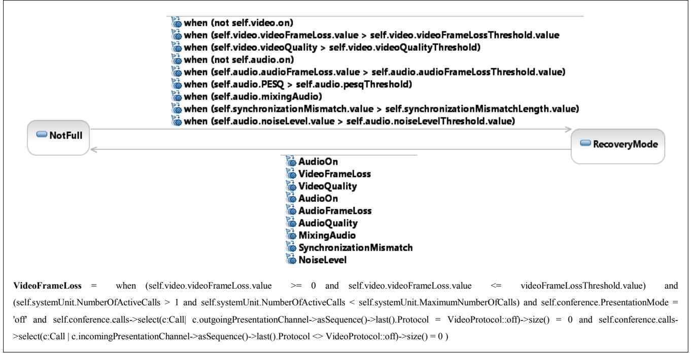
Figure 27. An excerpt of woven state machine obtained after applying the MediaQualityRecovery aspect
