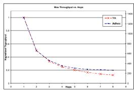
Fig. 3. Reference throughput vs. successive wireless hops
