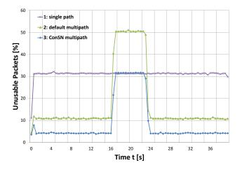
Fig. 6. Coupling WLAN and 3G Links (WLAN capacity too small)
