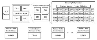
Figure 1. Nvidia GF100 Compute Architecture
