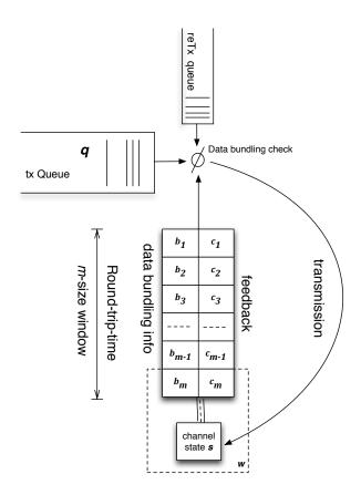
Fig. 1. SR ARQ and data-bundling Transmission Process
