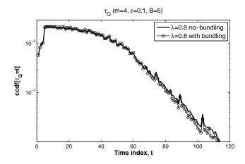
Fig. 5. Queueing delay  $au_Q$  with and without bundling,  $\lambda$  0.8, B=5, m=4,  $\varepsilon$ =0.1
