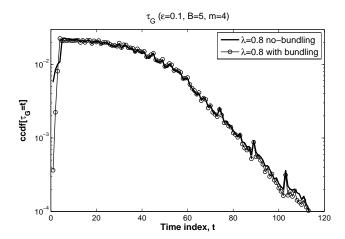
Fig. 7. Overall delay  $\tau_G$  with and without bundling,  $\lambda=0.8, B{=}5, \, m{=}4, \, \varepsilon{=}0.1$
